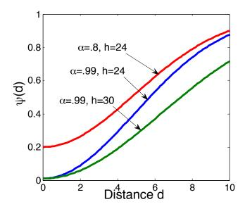
Fig. 3. The interaction potential  $1 - \alpha \exp(-\frac{1}{2h^2}d^2)$ , for various  $\alpha, h$ .
